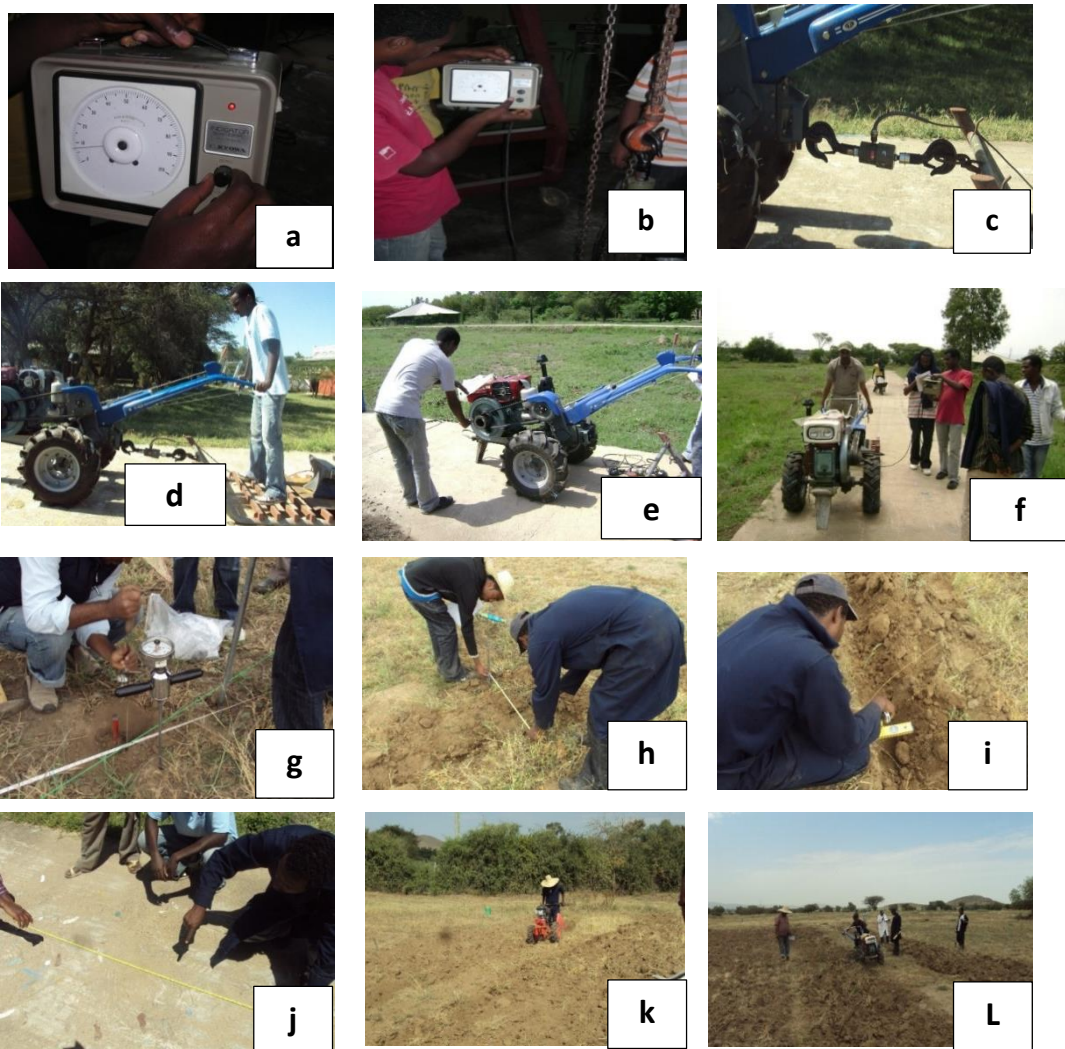
Figure 3 a) Analog indicator of drawbar force (left) and calibration of the load cell (right) before conducting testing b) Drawbar force measurement set-ups using dynamometer (left), Engine RPM measurement using digital non-contacting type tachometer( middle) and the load cell reading (right) on a concrete test track at Melkassa Agricultural Research Center (MARC) c) Soil shear and con-penetrometer reading (left), Ploughing width measurement (middle) and depth of tillage measurement (right) at Melkassa Agricultural Research Center (MARC) d) Slip measurement on concrete test track (left), DongFeng (DF-15) Chinese 2WT during testing (middle) and Vari brand Czech Republic made 2WT during testing at Melkassa Agricultural Research Center( Photo Source: Bisrat Getnet)
